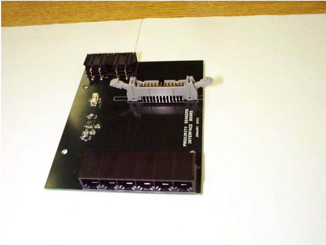
Fig. 1. The proximity interface board
