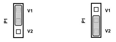
2. Admissible positions of shunts at the P1 switch are the following (any other position is prohibited):
