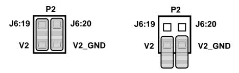
3. Admissible positions of shunt at the P1 switch are the following (any other position is prohibited):
